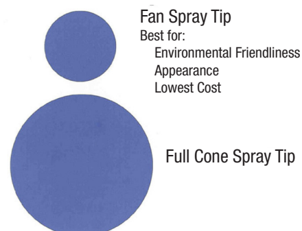
Figure 1: Relative Droplet Sizes - Magnified 30 Times
