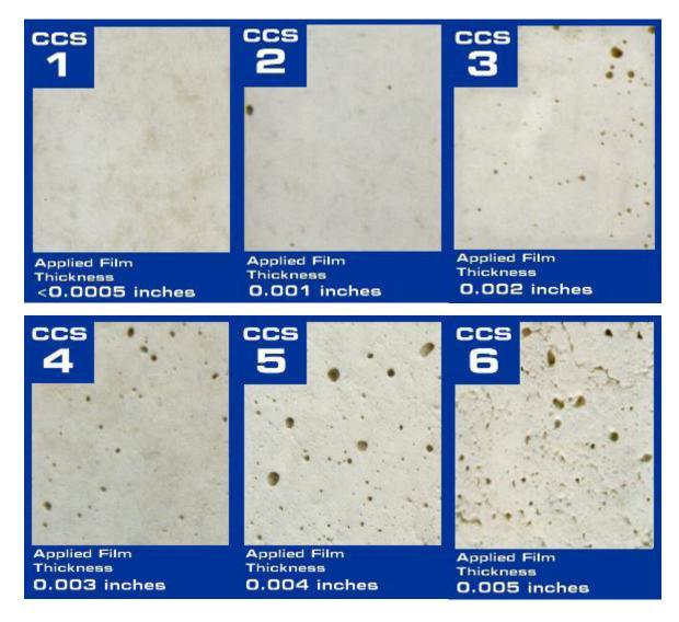
Suggestion: Take a picture of the 4 color printed version and hold next to the hardened concrete surface. You do not need to be present to evaluate the surface... just look at the picture.
